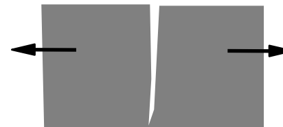
stress corrosion cracking
