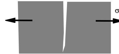
stress corrosion cracking
